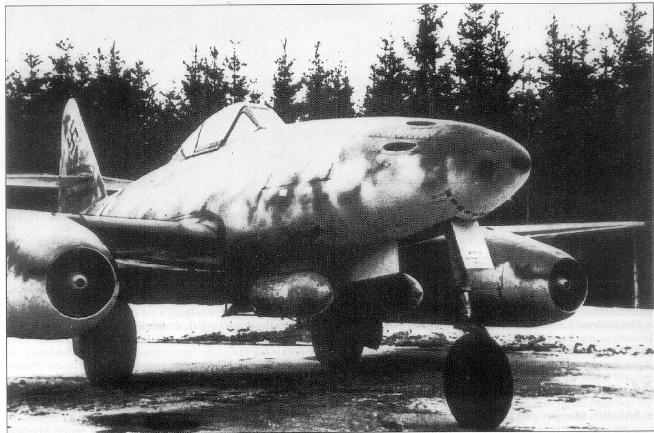
Me 262A-1a/Jabo se závěsníky "Wikingerschiff" a 250kg pumami. A Me 262A-1a/Jabo with "Wikingerschiff" bomb racks and underslung 250kg bombs.
